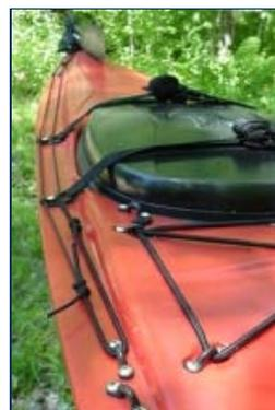
3/16 inch bungee. A rudder rest may be molded directly into the deck, or is a separate V shape fitting.
