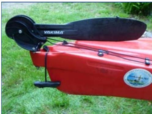
The Yakima Rudder Assembly (shown above is a circa 2003) has four screws side to side, One is large: the central pivot screw. Three are much smaller. All hold the two halves of the rudder housing together. Other version of the assembly should be very similar.
