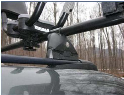
4. A variety of custom mounting options exist to secure sport rack crossbars to a vehicle roof. Usually this requires drilling holes into the roof and screwing base plates or tacks to the car top. This can be tricky work, sometimes best done at a body shop.
