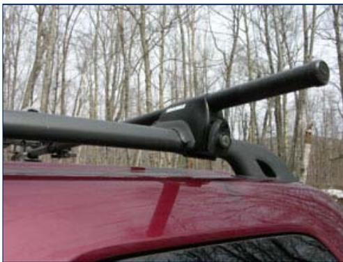
A two-door sedan may require a short roofline adaptor (SRA) in order to load long objects, such as paddle craft. The SRA propose is to place the rear bar further back on the car roof. A SRA is used with the doorframe style rack system. The front bar is located at the front of the doorframe. The SRA is a pair of bridges between the front and rear bars, above the doorframe. The clips hang off the SRA, grasp the doorframe, and hold the rear bar firmly in place.
