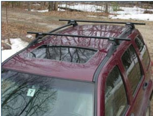
Essentially a sport rack is a pair of bars that span from side to side, supported by feet that bear the load to the car top. They are secured to the car in some fashion, often with a lock and key. Once the crossbars are in place you can add sport specific accessories to carry your water-sport, snow-sport or bike gear.
