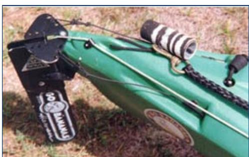
While the Scupper rudder assembly is robust the bungee cords are very likely to fail, and when they do so the rudder will not automatically deploy to the default position, straight down. There is a small chance of the lifting line requiring replacement too. The blade will rarely break, but may become bent and cracked. Bungee, lift line and blades are easy to replace. If one were to perform a rudder overhaul the anodized aluminum could be "repainted" at that time for cosmetic purpose.
