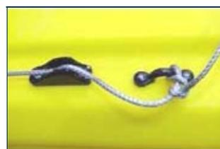
At this time you may wish to check your rudder control lines. Original Scupper rudder control line is a very strong string. These lines run internally through rudder cable tubes that poke out of the kayak at the stern end and in the cockpit sides. These strings can be replaced with any synthetic cordage that is very strong. I recommend that you replace the control lines with stainless steel rudder cables. To do so you will need a standard rudder cable kit, plus some thimbles and shackles.
