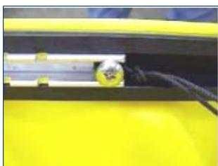
Standard Stainless steel rudder control cables have an eyelet on one end of the cable. This is often secured with a small nut and bolt, or a clevis pin and ring. In most cases the eyelet is secured to the wings of the rudder assembly.
