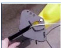
When finished, with the blade deployed in the down position, the lift line should start below the large nylon washers, come up on the stern side of one washer, up through the housing, through the open slot in the upper wing, directly over the pivot pin and then on toward the cockpit.
