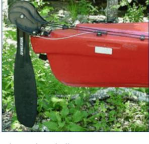
When crossing open water, wind, waves and currents will "push" your kayak around and a rudder blade can help keep the kayak straight, much like the feathers on an arrow allow it to fly true.
