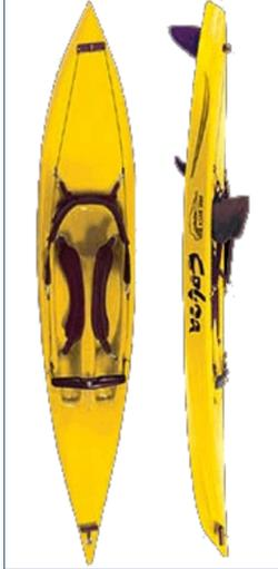
Some kayaks, mostly surf skis, will sport Through-Hull rudders that are mounted close to the stern, but not at the far end. Note the Cobra Wave Witch photo (left). They protrude from the bottom of the hull and have shaft that swivels in a tube that is through the hull. The top of the shaft has a T-bar that attaches to the cables on the top of the back deck. This is sometimes concealed by means of a cover plate.
