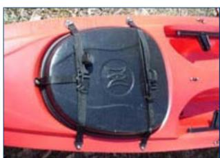
One of the more common hatch styles consists of a large plastic lid that is held fast to the deck and hatch opening by means of cargo straps. A gasket seals the hatch by filling the space between the lid and the deck. The gasket is attached to the lid, hatch rim or both. This article will focus on the hatches that have one or two gaskets and close by means of cargo straps. (See "[Alternative Hatch Styles](#)" below")
