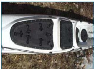
Some large style cargo hatches, like **Cobra's "A" hatch**, which can be installed on any kayak with a large, flat surface, have a very effective seal. This is accomplished by use of many toggles sealing a plastic lid, to a rim fitted with an O-Ring like gasket. While it does provide a very dry seal, the many toggles may appear to be daunting. No improvement is necessary on this style of hatch, except possibly a small "leash" to keep the plastic lid from getting lost.
