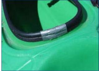
Cut it a little bit longer than it needs to be (about an inch or more) and that will ensure a good push-on fit with a tight seal. Trim with duct tape as necessary. For the most part you will use 1/2" inside diameter X 1 3/8" outside diameter size pipe insulation, do some careful measuring of length and diameter needed and assess the stock at your local hardware store for the best size and fit. (Tarpon hatch
