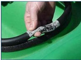
If only a few inches or two of the gasket is torn from the trim lock, glue can work, any more than that and you should get a replacement gasket or a roll of duct tape. If you do glue, have plenty of twist ties handy to hold the work together while the glue dries. You will have to remove the entire gasket from the kayak to work on it, leave plenty of time to cure before re-mounting it and use. (Photo: Repaired with Duct Tape)
