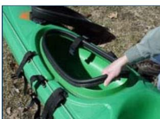
After a while a gasket will fail from age and over use. Fear not! You can get replacements from the kayak shop or the manufacture. Double check the make and model and make sure you are ordering and getting the right parts. (Photo: Trim lock gasket spare parts)
