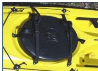
The system will not work if the neoprene cover is not in place, so double check to make sure the hatch is properly secure before launch. No improvement is necessary on this style of hatch, except possibly a small "leash" to keep the neoprene cover from getting lost.
