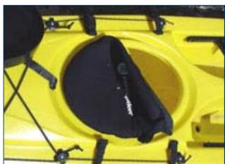
Other types of hatches will utilize a **Neoprene cover** stretched onto a combing encircling the hatch rim and closed with a plastic lid secured by straps. You will find this style on some Necky and Perception kayaks. While this system does seal very effectively, and keeps the inside quite dry, it can be hard to use. A smaller hatch size can inhibit loading, and stretching the cover can be troublesome.
