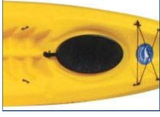
Many kayakers will be outfitted with a **Rubber Hatch Cover**. This type will snap onto a raised lip on deck, much like a Tupperware lid.
