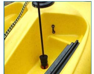
Some times an inner tube type flagpole mount can be used, with some extra strapping to and threaded through the scupper hole; but what if you your kayak does not have scupper holes? A pole with its own float can be tethered to the kayak if necessary, but there are other alternatives,
