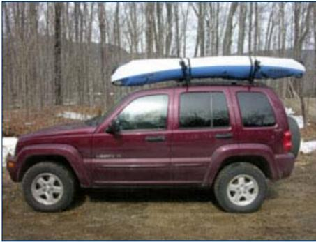
Recreational sit-in-side kayaks do not load well upside down, on the cockpit coaming. Loading them directly on crossbars, hull up, or down, will cause dents and deformation. They must be loaded on saddles or J-Cradles. Typically you will be able to load only two rec kayaks, sit-in and/or sit-on, per car, maybe as many as three, on wide cars, outfitted with J-Cradles. Even shorter kayaks should be secured, bow and stern, to the bumpers, when ever possible.
