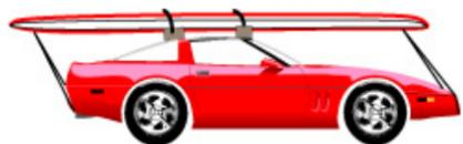
Extra long crossbars on skinny and low roof cars can cause trouble. Place bars away from locations where you are likely to stand up while exiting the car. Put day glow color tennis balls, or pool noodles, on the 4 ends of the crossbars to soften the blow and add visibility. If your bars really stick out allot, try to park well away from the path of pedestrians.
