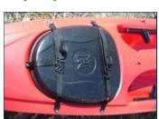
One of the more common hatch styles consists of a large plastic lid that is held fast to the deck and hatch opening by means of cargo straps. A gasket seals the hatch by filling the space between the lid and the deck. The gasket is attached to the lid, hatch rim or both. This article will focus on the hatches that have one or two gaskets and close by means of cargo straps. (See "Alternative Hatch Styles" below")
